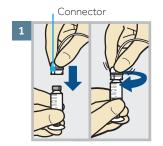
Gently push the tubing connector onto the reservoir. Turn the connector clockwise until locked. You will hear a click.
