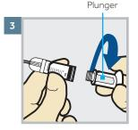
Twist plunger counter-clockwise to loosen and remove.
