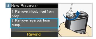
Remove the used reservoir from the pump.
