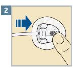
Gently hold the cannula housing steady with your finger. Then push the site connector straight into the cannula housing until you hear a click.
