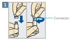
Gently push the tubing connector onto reservoir. Turn clockwise until locked. You will hear a click.
