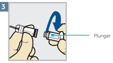
Twist plunger counterclockwise to loosen and remove.
